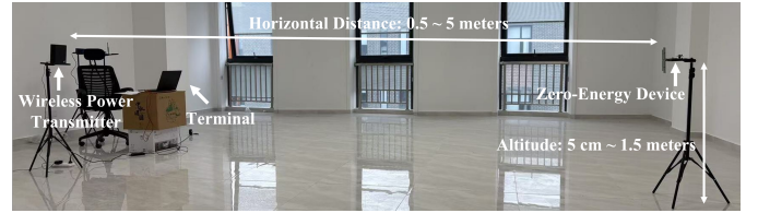
Fig. 7. Experimental analysis in LOS scenario across varying horizontal distances and altitudes.
