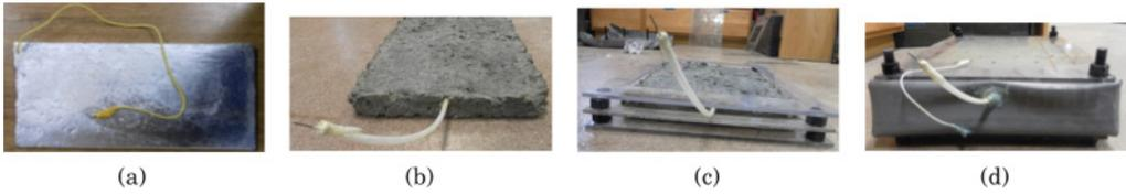
Fig. 6. (a) MFC's anode electrically connected to a copper wire. (b) MFC's cathode without the biofilm grown on it. (c) The cathode fixed by three polycarbonate sheets. (d) Assembled MFC wrapped by two rubber gaskets to prevent mechanical damages.
