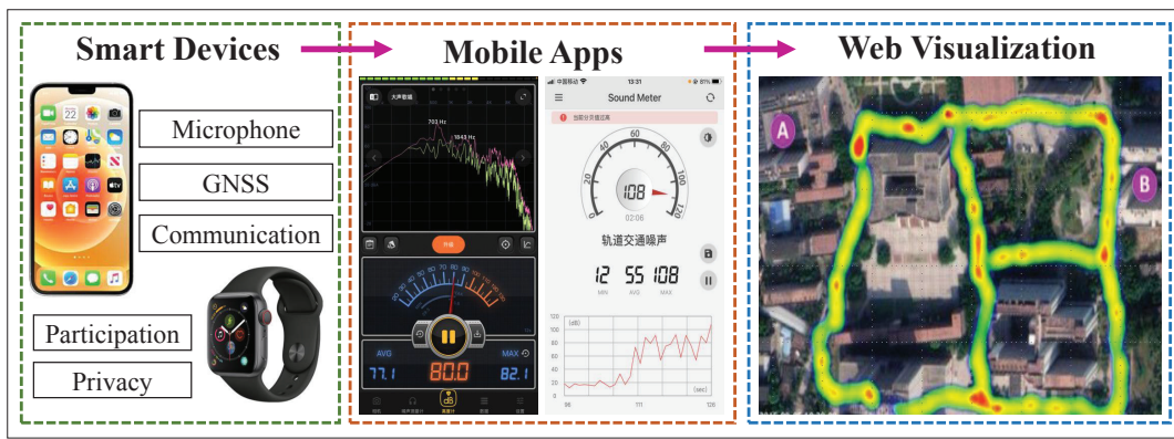
FIGURE 2. The technical principle of mobile noise crowdsensing.
